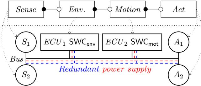
Figure 1: Control system architecture of a road vehicle.
