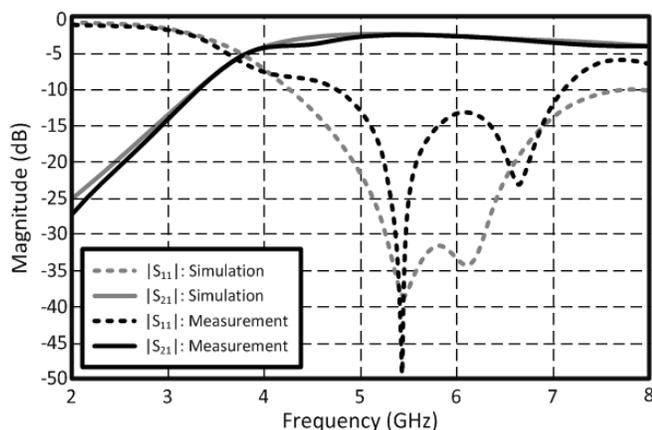
Fig. 15. Measured scattering parameters of microstrip-to-SIW transition.
