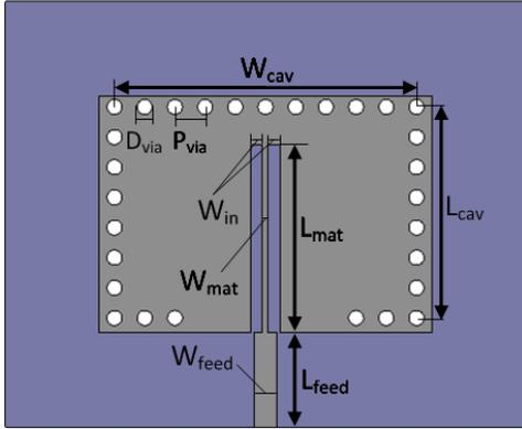
Fig. 12. Geometry of the SIW cavity resonator:  $W_{\text{feed}} = 2.5$  mm,  $L_{\text{feed}} = 10$  mm,  $W_{\text{cav}} = 32$  mm,  $L_{\text{cav}} = 22.4$  mm,  $D_{\text{via}} = 1.6$  mm,  $P_{\text{via}} = 3.2$  mm,  $L_{\text{mat}} = 17$  mm,  $W_{\text{mat}} = 0.6$  mm and  $W_{\text{in}} = 1.25$  mm.
