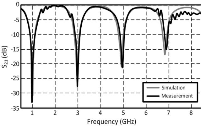
Fig. 3.  $S_{21}$  of the 1 GHz T-resonator.
