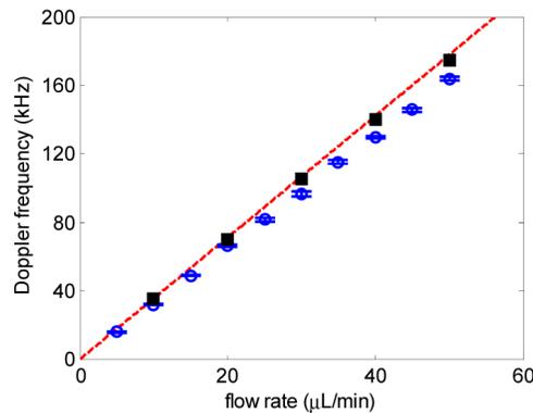
Fig. 11. Doppler frequency  $fd2$  profile versus different flow rates. The black solid markers and the blue hollow ones with error bars correspond to the simulated values and the measurement ones, respectively. The red dashed line is the calculation frequency curve associated with the maximal velocity values in channel center based on Eqs. (6) and (20).
