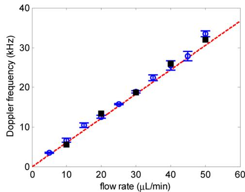
Fig. 10. Doppler frequency  $fd1$  trends as a function of the flow rate  $Q$ . The black solid markers correspond to the simulated values, and the blue hollow circles with error bars illustrate the measurement results. The red dashed line is the calculation result associated with the Fluent simulation velocity value in feedback power peak position in Fig. 6.
