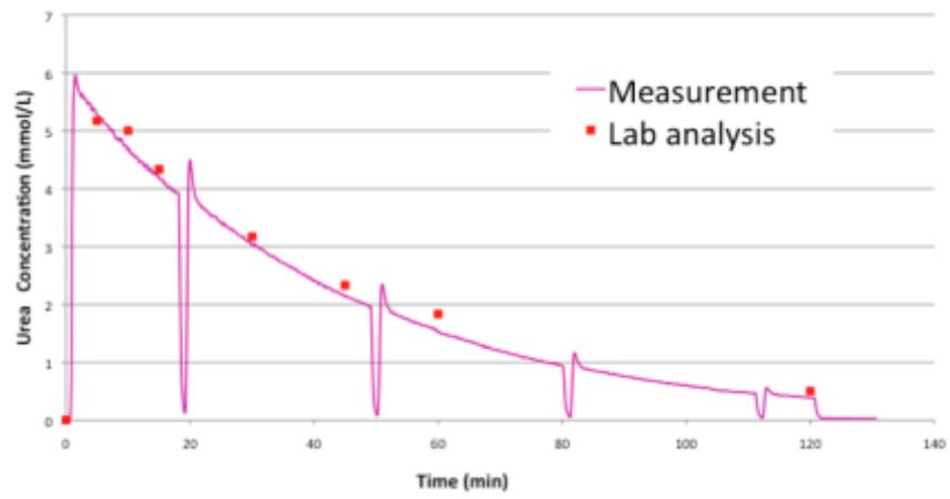
Figure 10: progress of urea concentration in dialysis conditions
