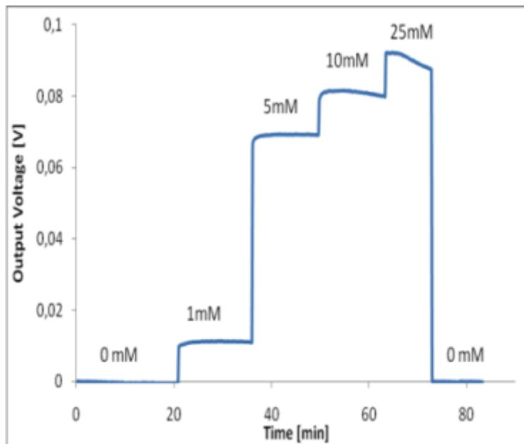
Figure 7: analytical response of urea in EDTA-based buffer solutions (pH = 7.4)
