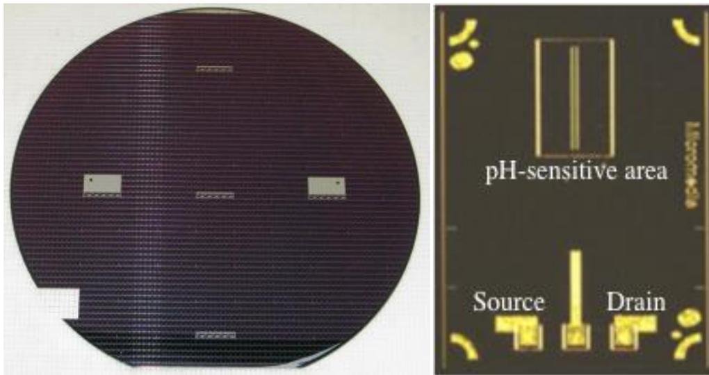
Figure 1: mass fabrication of pH-ChemFET chips (size: 2.1 x 1.6 mm<sup>2</sup>) in silicon foundry
