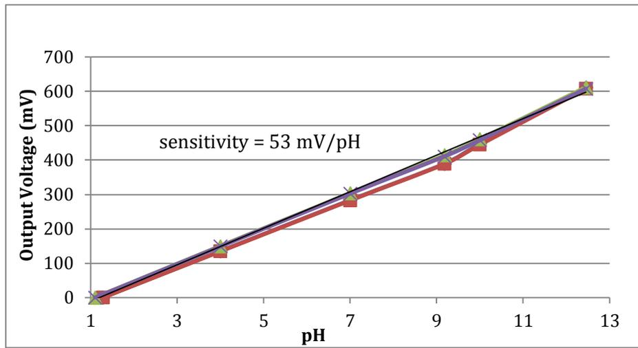
Figure 6: calibration curve of the pH-ChemFET microdevices
