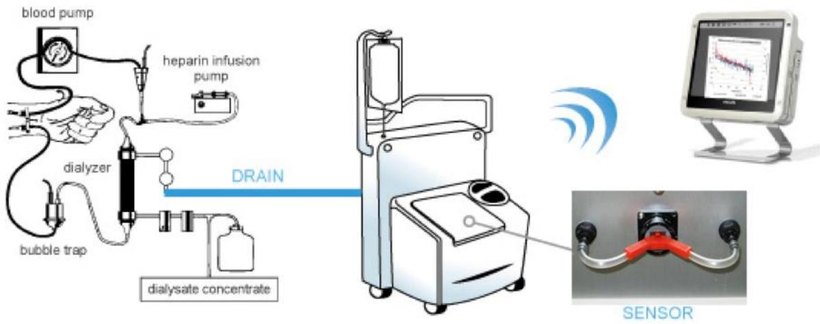
Figure 5: schematics of the urea on-line monitoring in dialysis conditions
