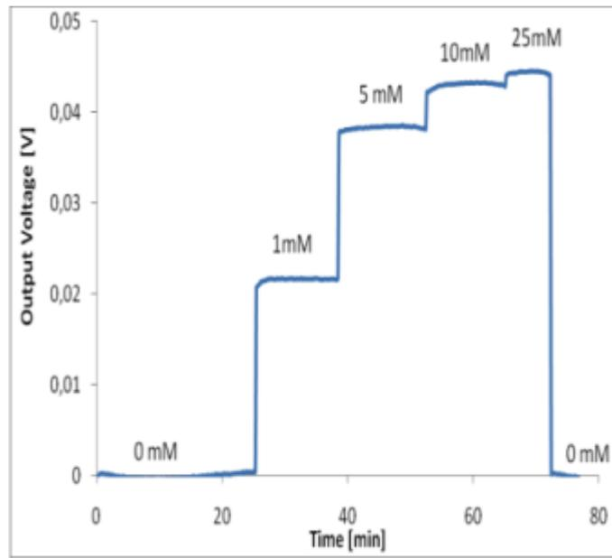
Figure 8: analytical response of urea in dialysate solutions (pH = 7.4)
