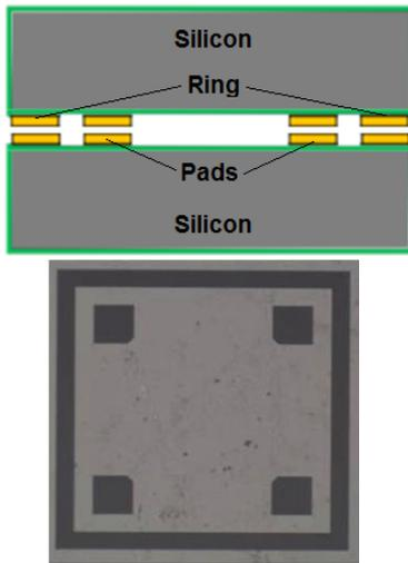
Figure 1: Test structure 1. Cross section & top view
