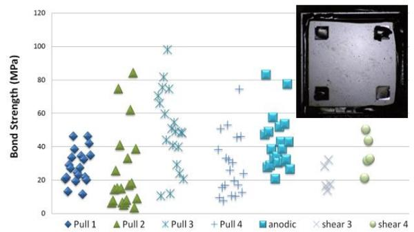
Figure 4: Cohesive fracture on silicon die and bond strength obtained with pull and shear tests
