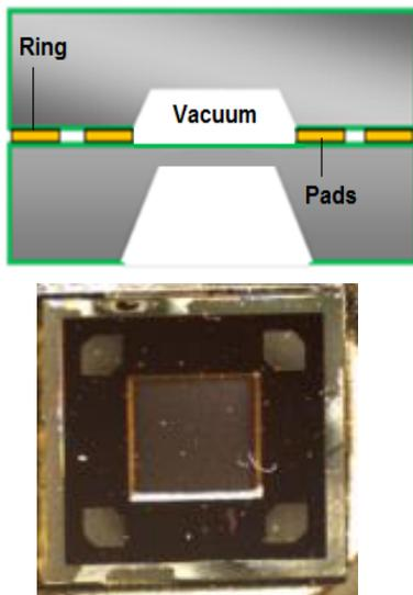
Figure 2: Test structure 2. Cross section & top view
