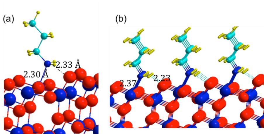
**Figure 8.** Most stable configurations obtained for PPA adsorbed on anatase (101) TiO<sub>2</sub> surface at a) 0.25 ML and b) 1 ML. Bond lengths are given in Å.
