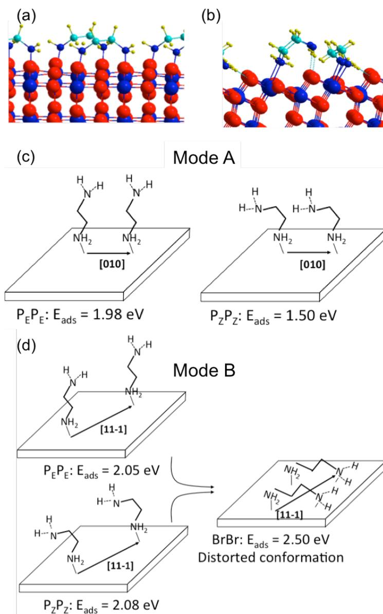
**Figure 4.** a) and b) Adsorbed configurations at 0.5 ML for isoenergetic *BrBr* and *BrP<sub>Z</sub>* structures, respectively. c) and d) Possible arrangement of DAE molecules on the anatase (101) TiO<sub>2</sub> surface at a coverage of 0.5 ML by considering only vertical adsorption *PP* modes (c), and path from perpendicular to parallel configurations (d), Mode A and mode B are significant of DAE molecules aligned in [010] and [11-1] directions respectively.
