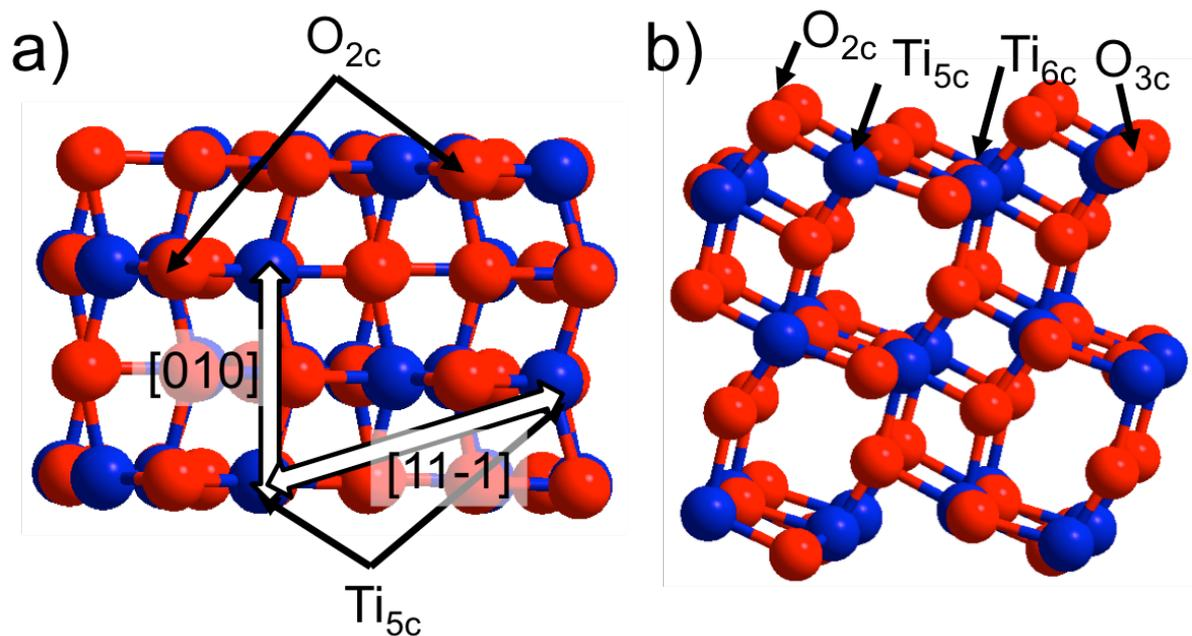
**Figure 1.** a) Top view and b) Side view of the periodic slab used to model the anatase (101)  $\text{TiO}_2$  surface. Covalence of the titanium and oxygen topmost surface atoms and the so-called ‘short direction’ [010] and ‘long direction’ [11-1] between  $\text{Ti}^{4+}$  atoms are shown. Blue and red balls represent titanium and oxygen atoms, respectively. This color scheme is used throughout the paper.
