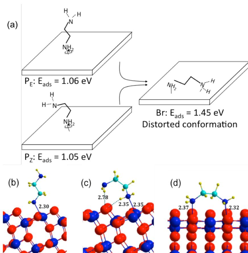
**Figure 3.** a) Possible orientations of the adsorbed DAE molecule on the dehydrated anatase (101) TiO<sub>2</sub> surface at 0.25 ML. The molecule lies parallel to the [010] direction. b-d) most stable structures. Bond lengths are given in Å.
