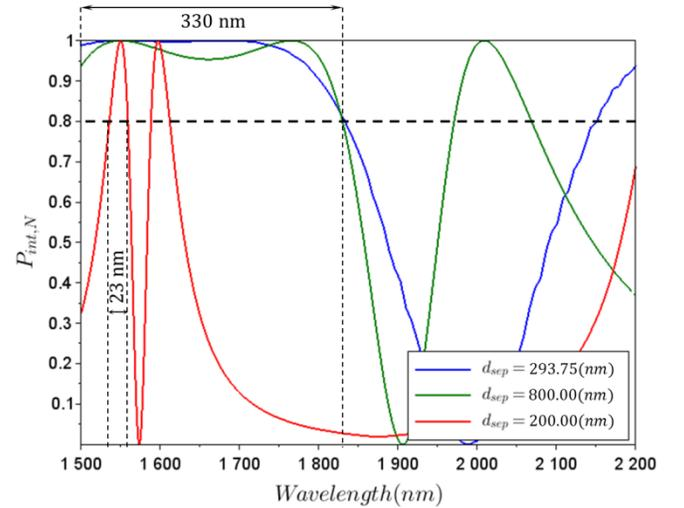
**Fig. 7.** Evolution of the normalized intra-cavity power  $P_{int,N}$  as a function of wavelength in (a) the PM case (red curve) with  $d_{sep} = 200.00 \text{ nm}$  and the PMM case at (b) optimal waveguide separation distance for scenario 1  $d_{sep} = 293.75 \text{ nm}$  (blue curve), and (c) optimal separation for scenario 2, at the cut-off separation distance  $d_{sep} = 800.00 \text{ nm}$  (green curve).
