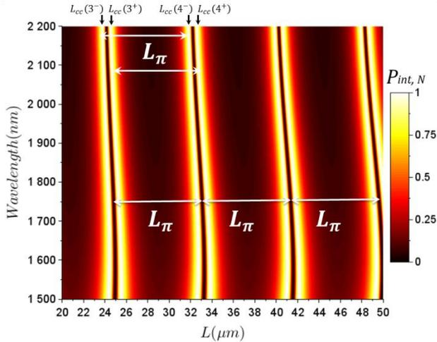
**Fig. 10.** Evolution of the normalized intra-cavity power as a function of coupler length and wavelength, in the PMM case for the optimal waveguide separation distance ( $d_{sep}=293.75$ nm). Here, the coupling orders correspond to  $m=3,4,5$ .
