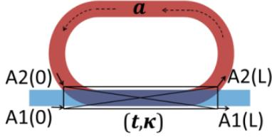
**Fig. 1.** Schematic of the studied vertically-coupled racetrack resonator.
