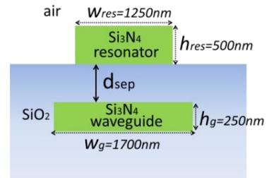
**Fig. 8.** Cross-section of the phase-mismatched racetrack resonator.
