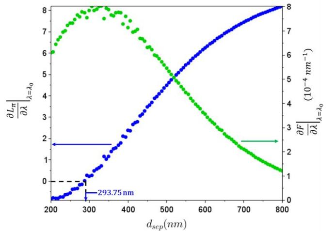
**Fig. 12.** Evolution of the chromaticity of the coupler beat-length  $L_\pi$  (left axis, blue dots) and of the power coupling efficiency  $F$  (right axis, green dots) as a function of the waveguide vertical separation distance  $d_{sep}$ .
