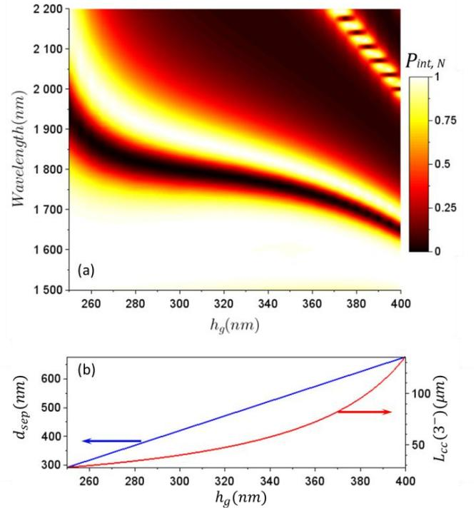
**Fig. 14.** (a) : evolution of the normalised intracavity power spectrum as a function of the access waveguide thickness  $h_g$  (resulting in a varying  $\delta^2$ ) for the achromatic- $L_\pi$  scenario. (b) : evolution of the separation distance at which the achromatic- $L_\pi$  scenario occurs (blue curve) and of the corresponding critical coupling length (red curve) as a function of the access waveguide thickness  $h_g$ .
