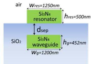
**Fig. 5.** Cross-section of the considered (quasi-)phase-matched racetrack resonator
