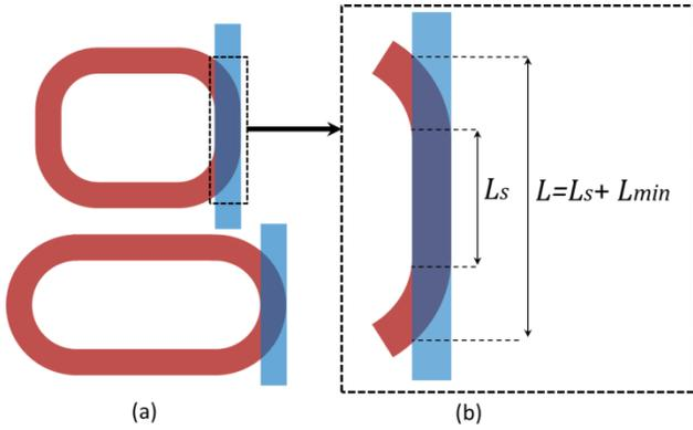
**Fig. 3.** Geometry of the vertically-coupled racetrack resonators under study showing (a) the resonator deformation permitting a variation of the coupling length while keeping constant the resonator loss and (b) a close-up view of the effective coupling length.
