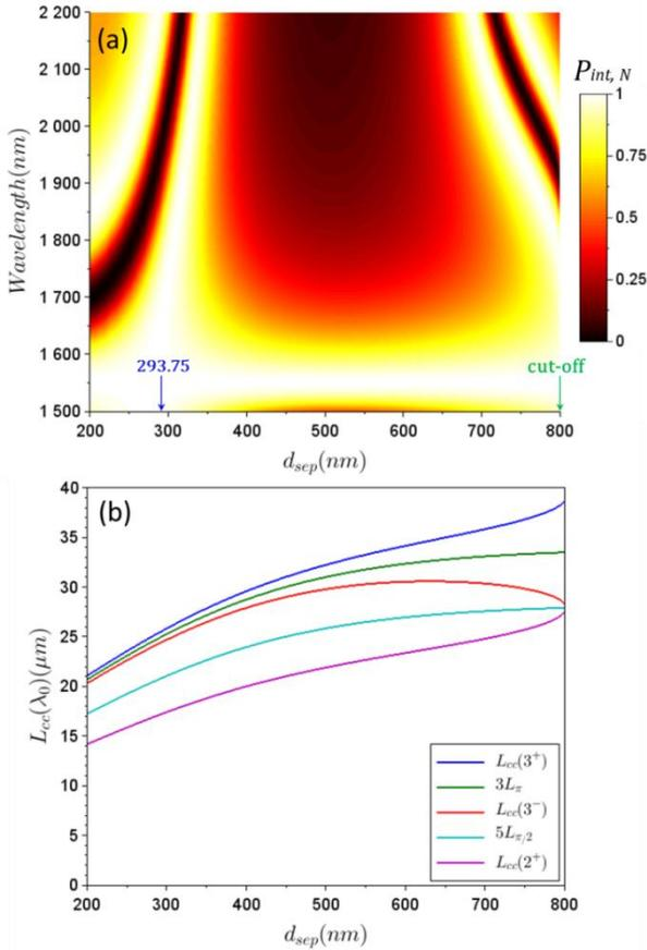
**Fig. 13.** (a) Evolution of the normalized intra-cavity power as a function of the waveguide separation distance and wavelength, in the PMM case for the critical coupling order  $m=3^+$ . (b) Evolution of selected critical coupling lengths and coupler characteristic lengths as a function of the waveguide separation distance.
