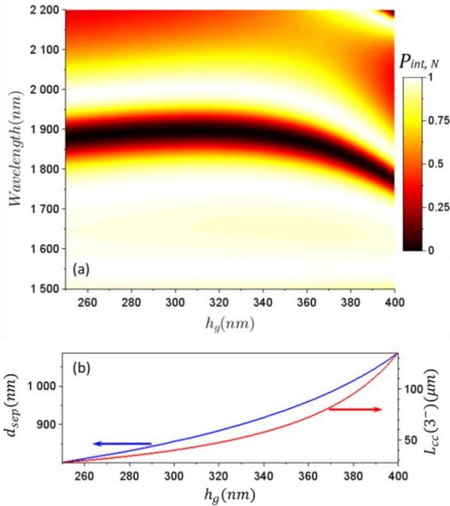
**Fig. 15.** (a) Evolution of normalised intracavity power spectrum as a function of the access waveguide thickness  $h_g$  (resulting in a varying  $\delta^2$ ) for the achromatic- $F$  scenario. (b) : evolution of the separation distance at which the achromatic- $F$  scenario occurs (blue curve) and of the corresponding critical coupling length (red curve) as a function of the access waveguide thickness  $h_g$ .
