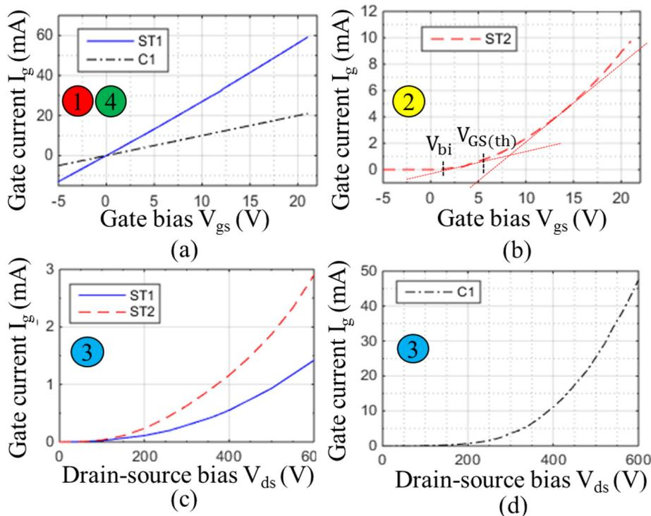
Fig. 6. Measurement results on damaged components. (a)&(b)  $I_C(V_{GS})@V_{DS}=0V$ . (c)&(d)  $I_C(V_{DS})@V_{GS}=0V$ .
