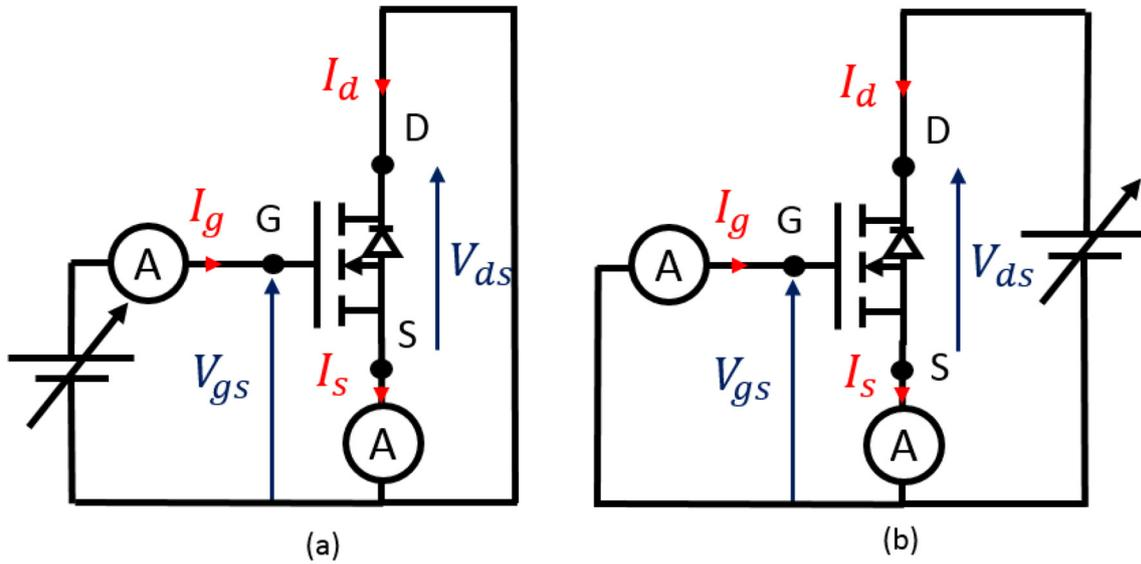
Fig. 5. Measurements performed with a SMU (Ref. Agilent B2902A 100fA 2ch.) and multimeter (Ref. Keithley 2700). (a)  $I_C(V_{GS})$  Measurement (b)  $I_C(V_{DS})$  Measurement.
