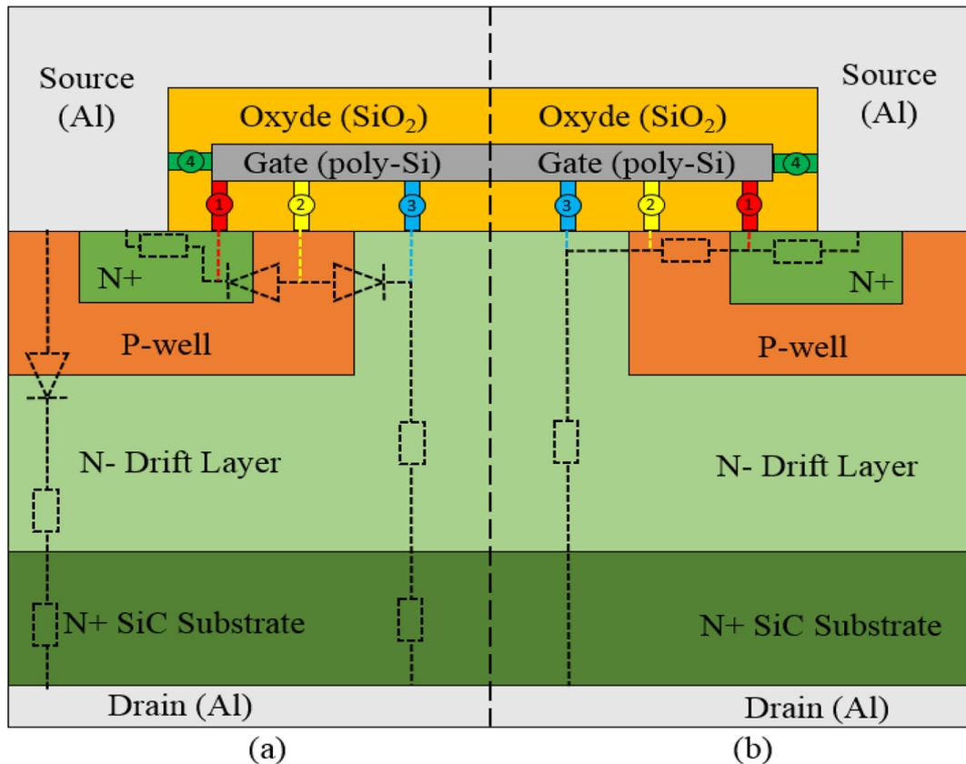
**Fig. 4.** Usual V-DMOSFET elementary cell. The local resistors named 1,2,3 and 4 models the damages in the oxide. (a)  $V_{GS} < V_{GS(th)}$ , the channel is non-conductive (b)  $V_{GS} > V_{GS(th)}$ , the channel is conductive.
