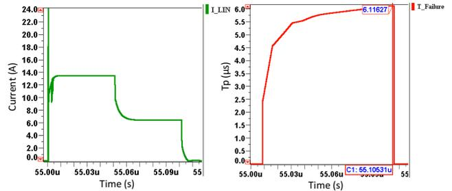
Fig. 14. Simulation LIN A under MR-TLP (400v)
