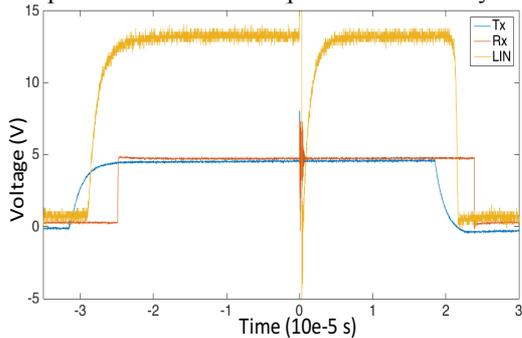
Fig. 8. Measurement results for the LIN C stressed by TLP (8A-300ns).
