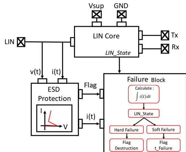
Fig. 1. LIN model behavior for failure investigation
