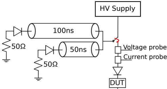
Fig. 13. Schematic of the MR-TLP
