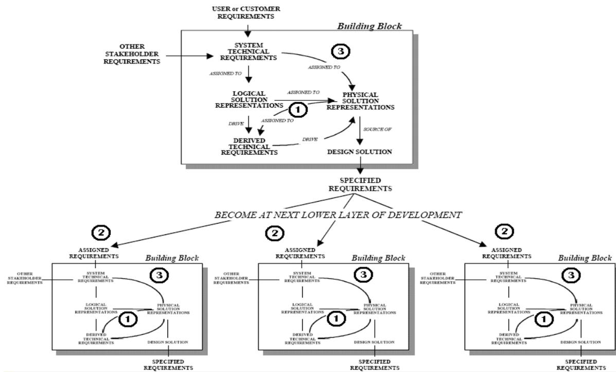
Figure 2. Architectural decisions using EIA632 System design process
