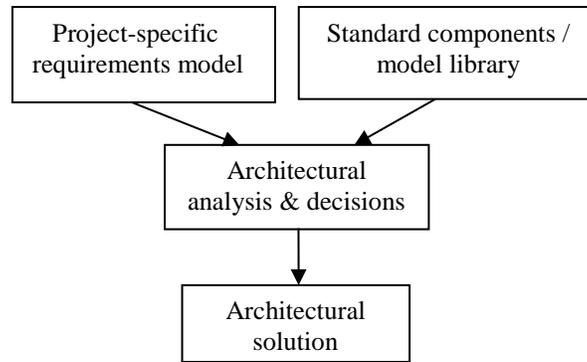
Figure1. A generic way to design system architecture
