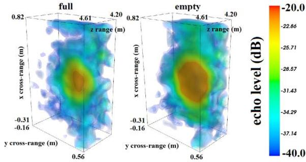
**Fig. 2** 3D representation of the microfluidic sensor echo when the gap is completely filled with water (left) or empty (right). The electromagnetic echo from the sensor antenna is not present in the 3D region considered in the Figure.
