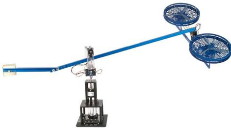
Figure 1: Picture of the Quanser “3 DOF Helicopter”.
