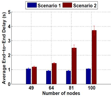
Fig. 3. End-to-end delay of Orchestra-based TSCH protocol, as a function of the number of nodes.
