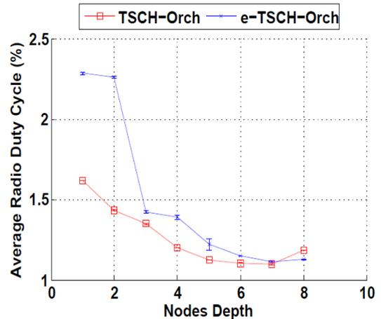
Fig. 12. Average duty cycle of TSCH-Orch and e-TSCH-Orch as a function of the nodes depth — The number of nodes is fixed to 64.
