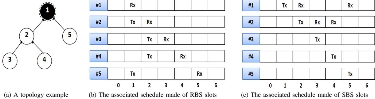
Fig. 2. Application schedule in Orchestra - illustration with a slotframe of length 7 time slots.
