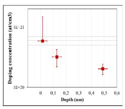
**Fig. 1:** Depth distribution of the active dopant concentration as determined by Differential Hall effect measurements from the SiGeOI sample implanted with Boron and laser annealed at an energy density of 0.68 J/cm<sup>2</sup>.
