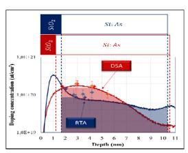
**Fig. 2:** Depth distribution of active dopant concentration for DSA and RTA processes measured by DHE (**colored dots**) compared to their respective SIMS (**colored lines**) from the 11 nm SOI samples implanted with arsenic at the same dose (10<sup>14</sup>at/cm²). Colored areas in the graph correspond to the active dose. Diagrams above graph zone represent the layers dimensions measured by ellipsometry.
