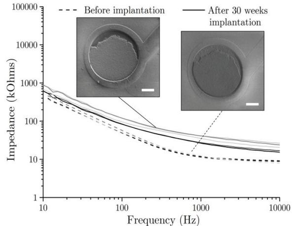
Fig 4. EIS evolution before and after 30 weeks implantation in mouse brain for PEDOT-modified electrodes, along with a representative SEM image before and after implantation (scale bar is 10 µm).
