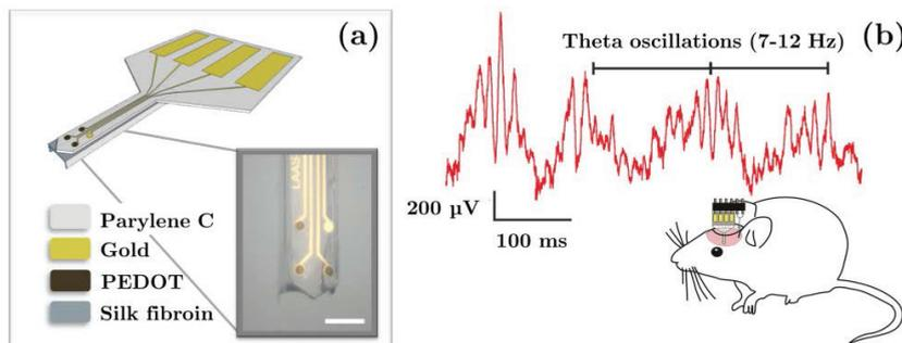
Fig 1. (a) Schematic representation (not to scale) and microscopic image (scale bar is 200  $\mu\text{m}$ ) of a Parylene C-based neural probe with three PEDOT electrodes and one gold electrode as control. The shank is supported on a resorbable silk coating to allow insertion in the brain. (b) Typical brain activity recorded from a freely-moving mouse discovering a new environment (acquisition cage). The Theta oscillations (7-12 Hz) are representative of an active behavior during exploration.
