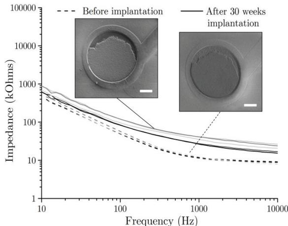
Fig 4. EIS evolution before and after 30 weeks implantation in mouse brain for PEDOT-modified electrodes, along with a representative SEM image before and after implantation (scale bar is 10  $\mu\text{m}$ ).
