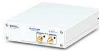
Figure 3. Picture of the USRP NI 2900
