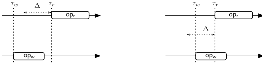
Fig. 1 Left: A write-latency-free read operation op_r . Right: a write operation op_w interfering with a read.
