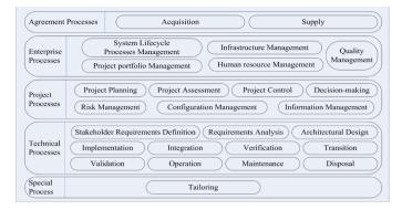
Fig. 2. Structure of the ISO/IEC-15288:2008 standard
