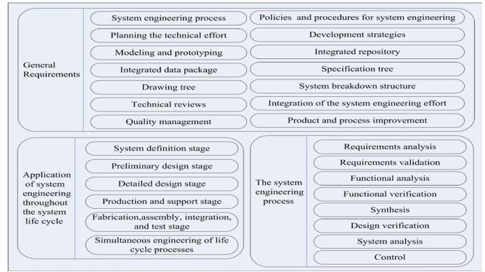
Fig. 3. Structure of the IEEE-1220:2005 standard
