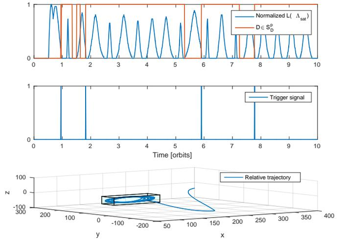
Fig. 1. Observed signals, trigger and controlled trajectories
