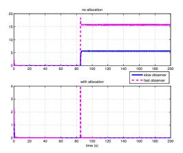
Fig. 6. Example 2: estimation error with and without allocation.
