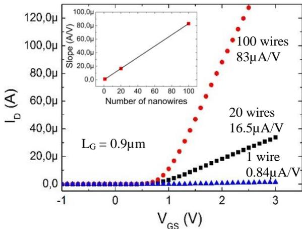
Figure 8:  $I_d(V_{gs})$  characterizations of Si-nw-MOSFETs, linear scale. ( $V_{ds} = 0.1V$ )
