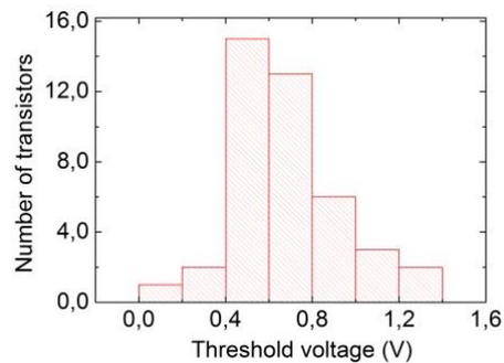
Figure 6 : distribution of the threshold voltage of the Si-nw-MOSFET.
