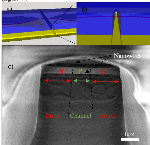
Figure 4: a) and b) schematic views of the Si-nw-ChemFET and the microfluidic channel. c) SEM view of suspended silicon nanowires inside a covered microfluidic channel (tilt 52°).
