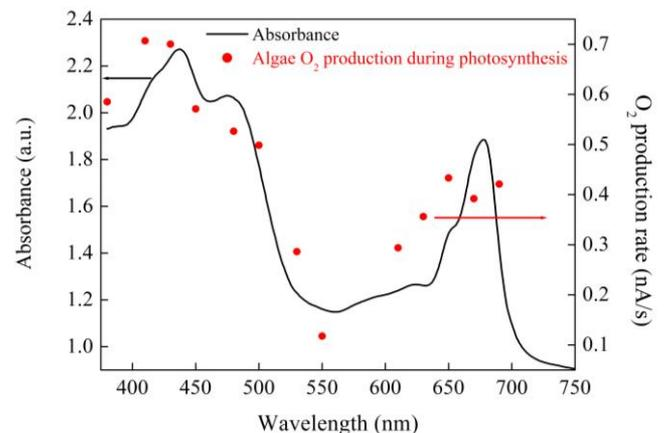
Figure 1. *Chlamydomonas reinhardtii* absorption spectra in High Salt Medium with the adjusted pH 6.8. and O<sub>2</sub> production during photosynthesis at different excitation wavelengths.
