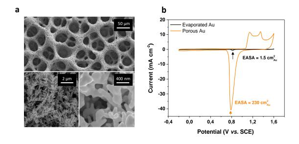
**Figure 2.** Characterization of the porous Au/RuO<sub>2</sub>.xH<sub>2</sub>O electrode. a) SEM images (top-view and cross-section) of the electrode obtained after 300 cycles of RuO<sub>2</sub> electrodepostion. b) Corresponding CV at 0.1 mV s<sup>-1</sup> in de-aerated 0.5 M sulphuric acid electrolyte. c) Determination of the outer capacitance ( $C_0$ ) of the electrode. d) Determination of the total capacitance ( $C_1$ ) of the electrode.
