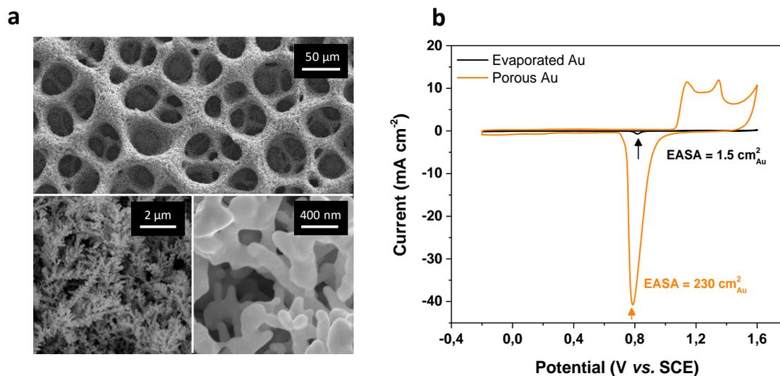
**Figure 2.** Characterization of the porous Au/RuO<sub>2</sub>.xH<sub>2</sub>O electrode. a) SEM images (top-view and cross-section) of the electrode obtained after 300 cycles of RuO<sub>2</sub> electrodeposition. b) Corresponding CV at 0.1 mV s<sup>-1</sup> in de-aerated 0.5 M sulphuric acid electrolyte. c) Determination of the outer capacitance ( $C_o$ ) of the electrode. d) Determination of the total capacitance ( $C_t$ ) of the electrode.
