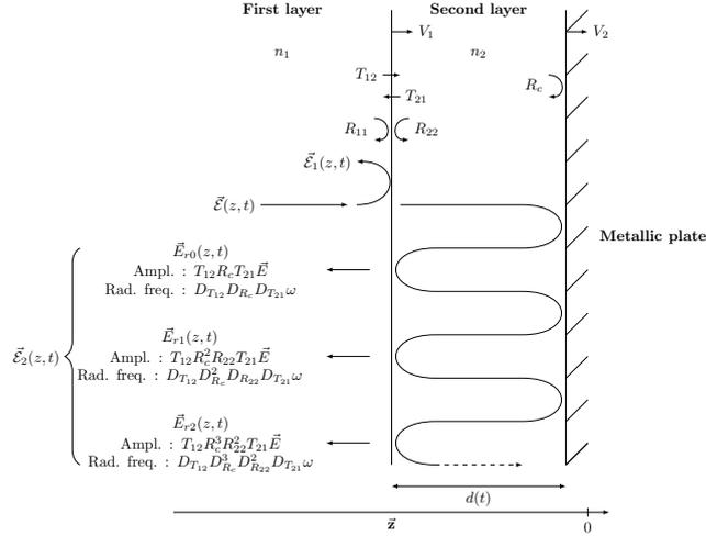
Figure 1: Configuration at time  $t$  with two moving interfaces: interface 1 (dielectric) and interface 2 (metallic) moving at constant velocities  $V_1$  and  $V_2$  respectively. At time  $t = 0$ , the two interfaces are located at  $z = 0$  and consequently, the separation distance  $d(t)$  between the two interfaces is given by  $|V_1 - V_2|t$ .
