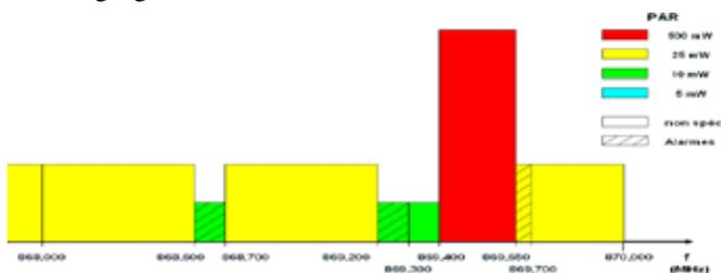
We use a statistical frequential repartition to choose one frequency that will have the emitted signal. More precisely, inside each channel of 200 kHz which is centered on  $f_c$ , the emitted signal will have a frequency that is far by  $f_i$  from  $f_c$ . The bandwidth of each emitted signal is around 100Hz which represents number of symbol bits emitted.
