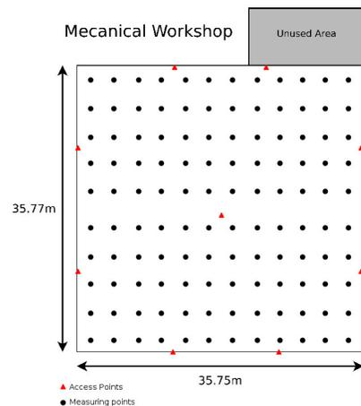
Fig. 2: Schematic of the workshop and measuring points
