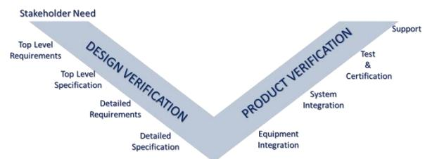
Figure 1 : System V cycle
