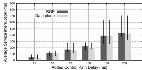
Figure 1: The dependency between control and data plane.
