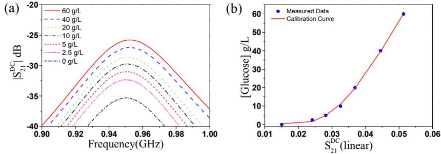
Fig. 2. Cross-mode insertion loss for different values of glucose concentration (a), and variation of the glucose concentration with the maximum value of  $S_{21}^{DC}$  (b). The calibration curve is depicted in (b).
