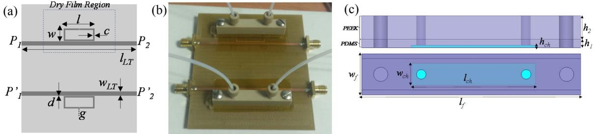
Fig. 1. Layout of the sensor metallic pattern (a), photograph of the fabricated device (b) and lateral and top views of the mechanical and fluidic parts (c). Dimensions are (in mm):  $w = 8.17$ ,  $l = 20$ ,  $c = 1$ ,  $d = 0.2$ ,  $g = 0.2$ ,  $l_{LT} = 75$ ,  $w_{LT} = 2.98$ ,  $h_1 = 3.5$ ,  $h_2 = 9$ ,  $w_f = 11$  and  $l_f = 50$ .
