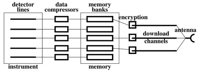
Figure 2: How data is produced, recorded, and downloaded.
