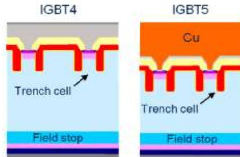
Fig. 2. Schematic of trench IGBTs
