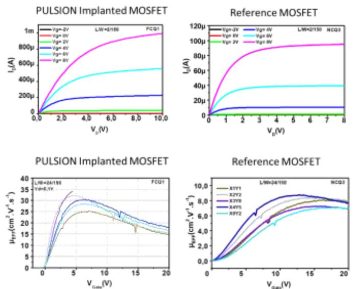
Fig. 6. Compared forward characteristics and extracted max. effective mobility of SiC MOSFET transistors with 2 $\mu\text{m}$  channel length : PIII implanted devices show a Drain current about 7x higher than reference devices for the same Drain and Gate voltages explained by a higher channel mobility.
