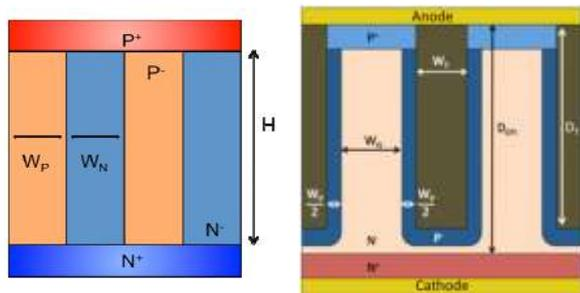
a-Schematic of a diode with standard EPI superjunction structure
