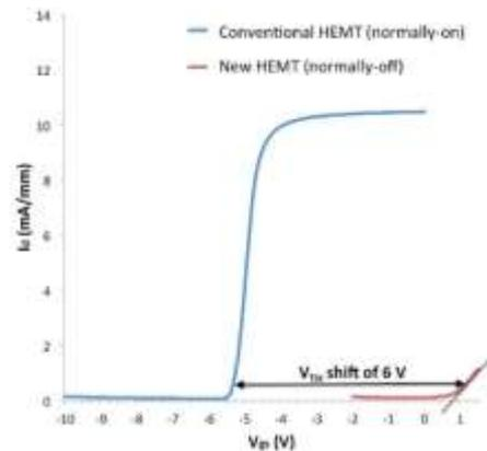
Fig. 10. Experimental transfer characteristics  $I_d(V_{gs}) @ V_{ds} = 1 V$  for the conventional normally-on HEMT and the new HEMT: 1st demonstration of a normally-off GaN HEMT thanks to PIII doping.
