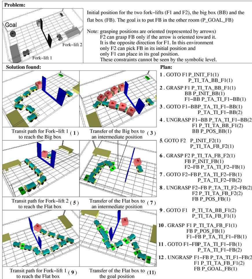
**Fig. 2.** Example of two fork-lifts ( F1 and F2 ) that have to carry the Flat box FB in the other room. The top figure shows the environment and the initial and goal positions. The second part shows the solution plan that has been produced by aSyMov (12 steps). Robots trajectories are illustrated in the left part.
