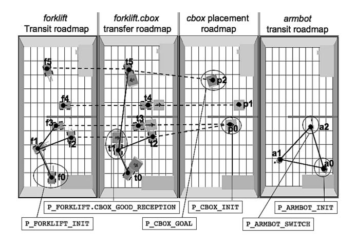
Figure 4: Roadmaps developed for the *radio-switch* problem. We also indicate the considered *place* propositions.
