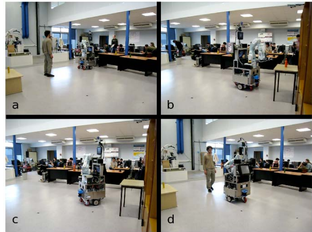
Figure 9. First PSP for known objects, approaching to the table, a) Initial position, b) Final configuration looking at the table. Second, PSP for humans, c)-d) Initial and final configuration looking at human
