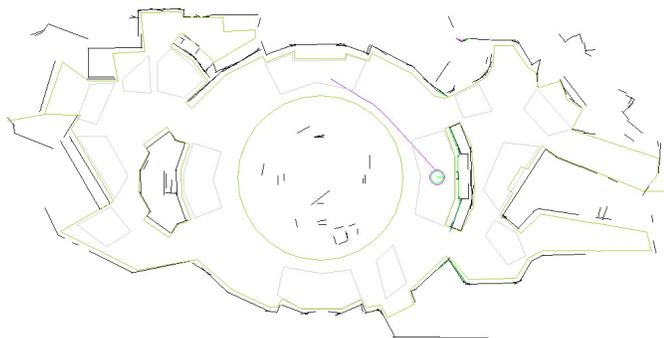
Fig. 4. The map of the environment built by Rackham contains 232 segments (black). It has been augmented with virtual obstacles (green or dark-grey) and target zones (light-gray).
