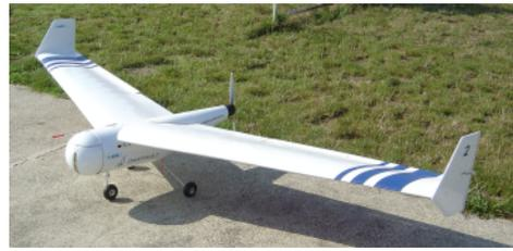
Fig. 8. The UAV Lhasa (3.0 m wingspan, 6.0 kg total)
