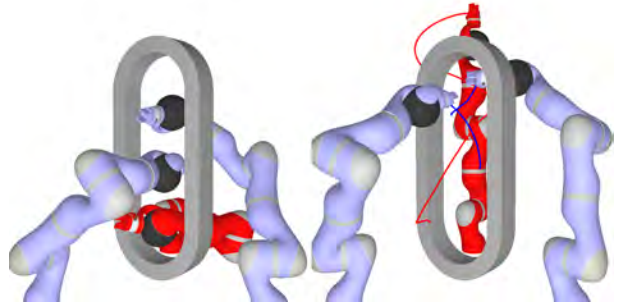
Fig. 1. Multi-robot costmap planning problem : initial and goal configurations of the active arm (red) and solution path that minimizes end-effector's displacements of the two passive arms (blue) hindering the path to the goal.
