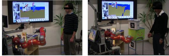
Figure 10: The human aware manipulation planner is able to handle free (left) and cluttered (right) environments.
