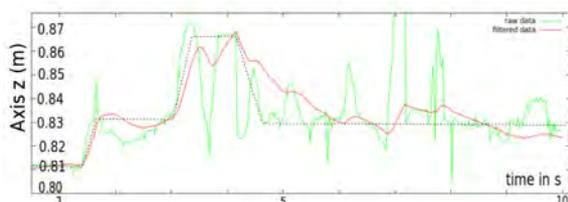
Figure 10: Instability of the 3D vision in poor lighting condition. The green curve shows axis  $z$  of the localization result of an object in the robot frame over 10 seconds and the red one shows the filtered result. The object was held by a human that intended to move the object accordingly to the black dashed curve.
