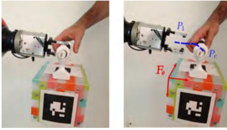
Figure 5: A simple case of grasp. Left: a planned grasp defines contact points between the end effector and the object. Right: To finish the grasping, the manipulator must follow the blue trajectory  $P_1 - P_c$ , and then close the gripper. This movement must be controlled in the object frame  $F_o$ .
