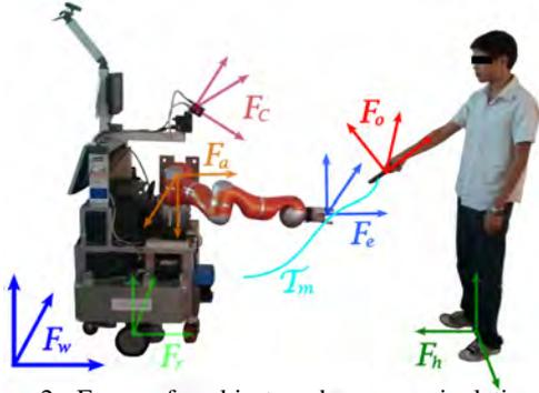
Figure 2: Frames for object exchange manipulation:  $F_w$ : world frame;  $F_r$ : robot frame;  $F_c$ : camera frame;  $F_e$ : end effector frame;  $F_o$ : object frame;  $F_h$ : human frame. The trajectory realizing a manipulation should be controlled in different task frames.
