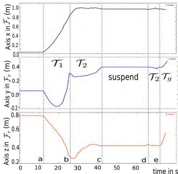
Figure 13: Real position of the robot arm end effector in the robot frame. The motion starts at time  $a$ ; Between  $a$  and  $b$ : the controller tracks the first trajectory segment  $\mathcal{T}_1$  in  $\mathcal{F}_r$ ; From  $b$  to  $c$  and  $d$  to  $e$ : target tracking; From  $c$  to  $d$ : the task is suspended; From  $e$  to end: the grasping movement controlled in  $\mathcal{F}_o$ .
