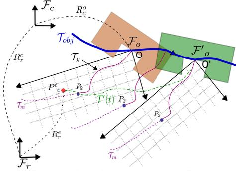
Figure 9: *Control Mode 2*. control mode. Object at time  $t_1$  is colored in light brown, and green at time  $t_2$ . It follows a movement model given as the blue trajectory  $\mathcal{T}_{obj}$ . The purple trajectory for grasping  $\mathcal{T}_g$  stays unchanged in the object frame. The robot tracks the trajectory  $\mathcal{T}_g$  as it does the grasping movement.
