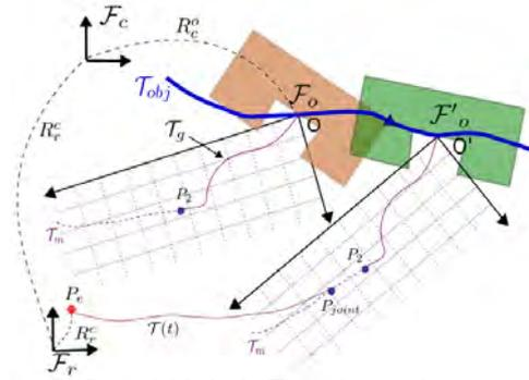
Figure 8: *Control Mode 1.* The robot tracks a point. The object moves to the right, it is drawn at two times: firstly in brown for time  $t_1$  and then in green at time  $t_2$ . In both cases, the entry point  $P_2$  of the trajectory  $\mathcal{T}_g$  is drawn relatively to the object frame  $\mathcal{F}_o$ .
