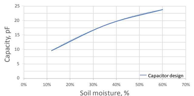
Fig. 3 : Capacity response of the capacitor design
