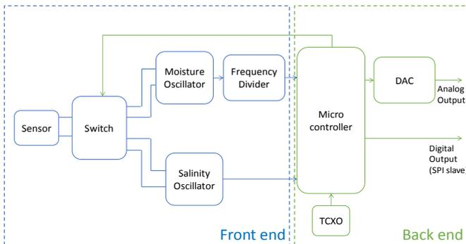
Fig. 8. Electronic architecture
