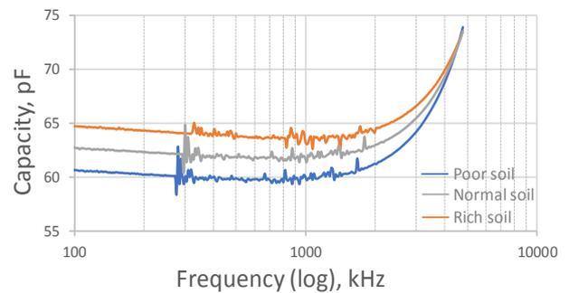
Fig. 5. Capacity according to the salinity
