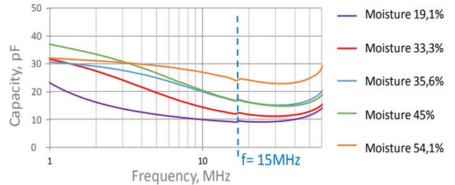
Fig. 6. Capacity according to moisture
