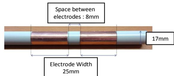
Fig. 2. Optimized capacitor design
