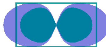
Fig. 2. Layout of the FDAs without rectangular metallic ring (purple) and with the rectangular ring (turquoise blue). The two antennas share the same lower frequency and gain.
