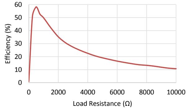
Fig. 8 Efficiency (%) as function of the load resistance for the FDR with a reflector positioned at 2.7 cm behind the rectenna (incident power density:  $S=33.9 \mu\text{W}/\text{cm}^2$ , frequency:  $f=3.25 \text{ GHz}$ )
