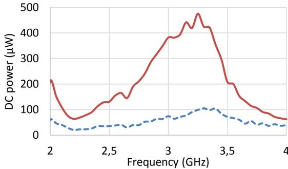
Fig.6. Measured DC power ( $\mu\text{W}$ ) for the FDR (incident power density:  $S=33.9 \mu\text{W}/\text{cm}^2$ , load  $1.5 \text{ k}\Omega$ ) as function of the frequency: dotted blue curve (without any reflector plane), continuous red curve (with a metallic reflector positioned at 2.7 cm behind the rectenna)
