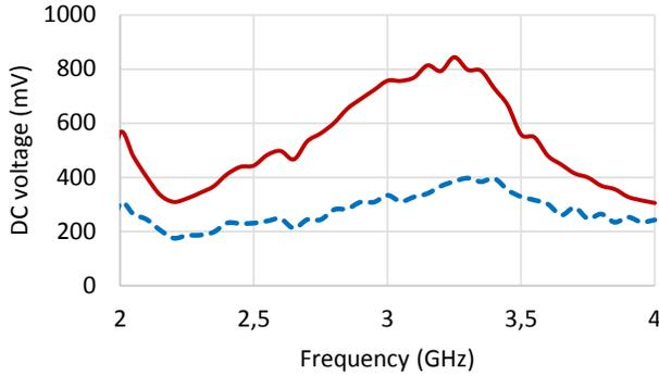
Fig.5. Measured DC voltage (mV) for the FDR (incident power density:  $S=33.9 \mu\text{W}/\text{cm}^2$ , load  $1.5 \text{ k}\Omega$ ) as function of the frequency: dotted blue curve (without any reflector plane), continuous red curve (with a metallic reflector positioned at 2.7 cm behind the rectenna)
