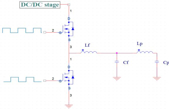
Fig. 7. Tx SPICE electronic circuit of the WPTS
