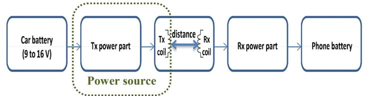
Fig. 1. Schema of a typical inductive WPTS
