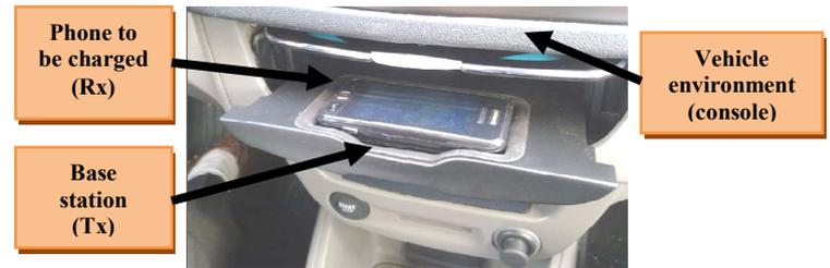
Fig. 2. Illustration of a WPTS in a vehicle environment
