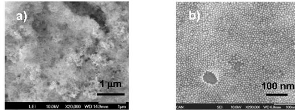
Figure 6: SEM images of a) highly porous 1 micron thick tin dioxide layer made of 20 nm large nanoparticles ( $G=x20'000$ ), and b) zinc oxide nanoparticles thin layer deposited on silicon substrate ( $G=x200'000$ ).
