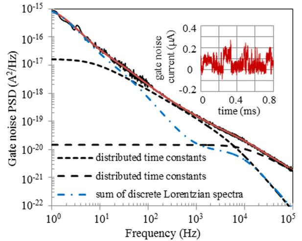
FIG. 4. Gate noise power spectral density versus frequency at  $V_R = 2.25$  V showing the different components of the model. The inset represents the variations of the gate noise current in the time domain and clearly shows the presence of burst noise in the device.
