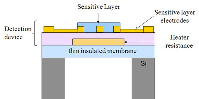
Figure 1: Structure of gas sensor.
