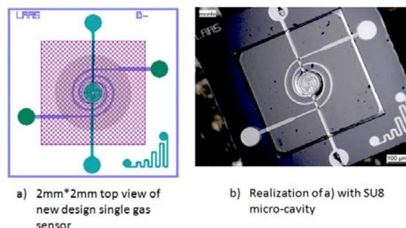
**Figure 6: Single gas sensor with SU8 micro-cavity.**
