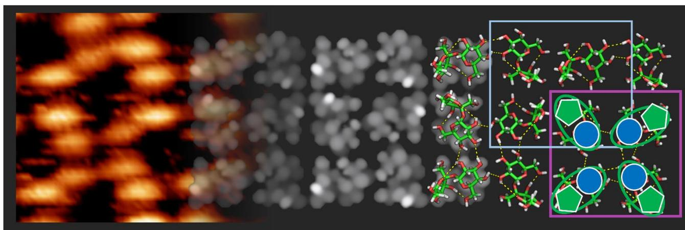
**Figure 3:** Model of the sucrose assembly pattern. Comparison of the measured STM image (left side) with the simulated STM image (center) demonstrating good qualitative agreement of the observed features, such as a porous structure and different intensities between the glucose (darker) and fructose (brighter) building block. On the right side, the molecular structures are presented, hydrogen bonds are indicated as yellow dotted lines.
